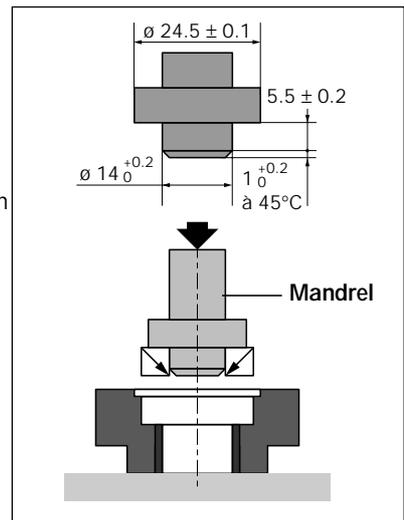
Using a press or a hammer, the seal is inserted in its housing.
