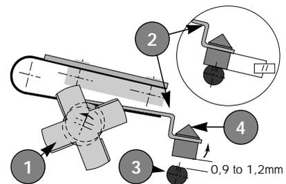
The stop valve face must be perpendicular to the axis of the oil inlet hole; when free, the stop valve should rest on its seat: check the parallelism of the lever in relation to the bearing face of the stop valve seat. Orient the seat to obtain the correct setting.
