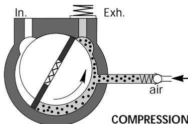
At the end of "compression", the pressure in the exhaust chamber is greater than atmospheric pressure. An anti-suckback device (valve + spring) prevents the gases and oil from being drawn back into the inlet.
