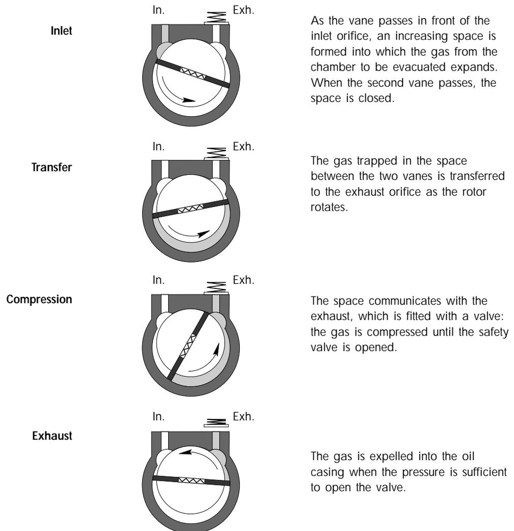
**Application** Single stage rotary vane pumps are the best choice for continuous pressures above 1.0 Torr (1,3 mbar), as well as applications where large amounts of condensable gases are present.
