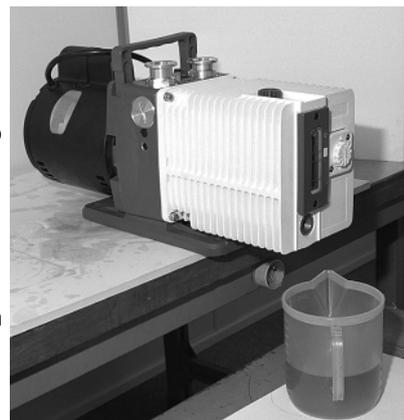
**Flushing** The draining operation can be followed by a flushing operation if the oil is particularly dirty. This operation requires a volume of oil equal to the capacity of the pump.
