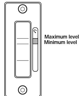
Note: Optimum pump performance and service life are obtained when the oil level is between the maximum level and the minimum level.
